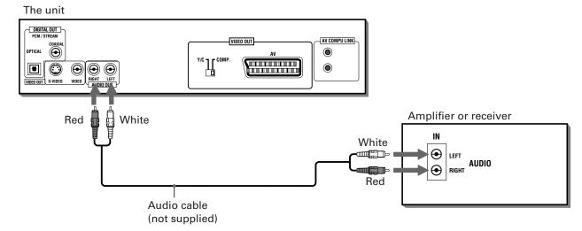
Connect the unit's AUDIO OUT to any line-level inputs (such as AUX, DVD, CD, etc.) of an audio amplifier or receiver.
